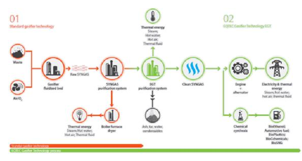
On average the number of cleaning processes varies between 7 and 10 steps, although it depends on the material used for the reaction and the end purpose. The complete cleaning purification process is called "synthesis gas purification system" (Syngas). The Syngas system is what makes Ebioss' plants unique and far ahead of the competitor proposition.
